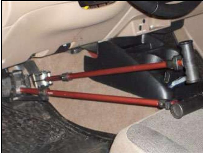
Peddle Master is designed to give disabled people the ability to drive their vehicles on their own. As long as they have access to a vehicle with an automatic transmission, they can get behind the wheel and hit the road. The Peddle Master can control the brake and gas pedals, and it's affordable and easy to transport.
